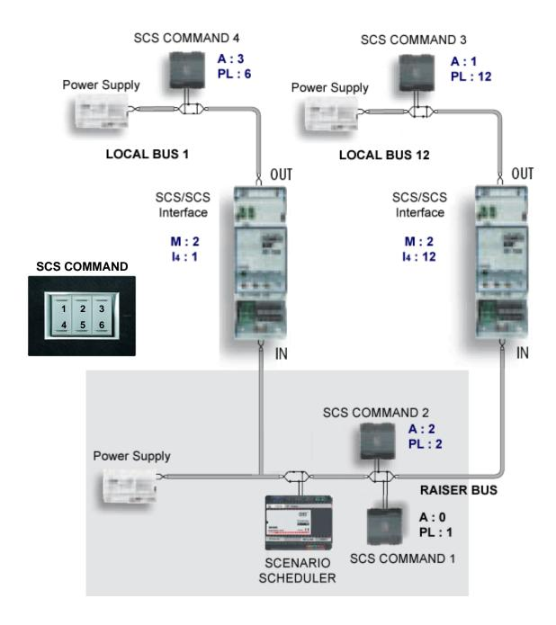
When the push button n° 1 of SCS Command 1 is pressed, keep pressed, then released an Open Web Net Client reads the following sequence of OWN Frames:
