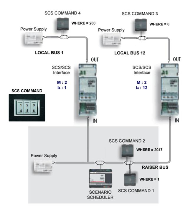
When the push button n° 1 of SCS Command 1 is pressed, keep pressed, then released an Open Web Net Client reads the following sequence of OWN Frames:
